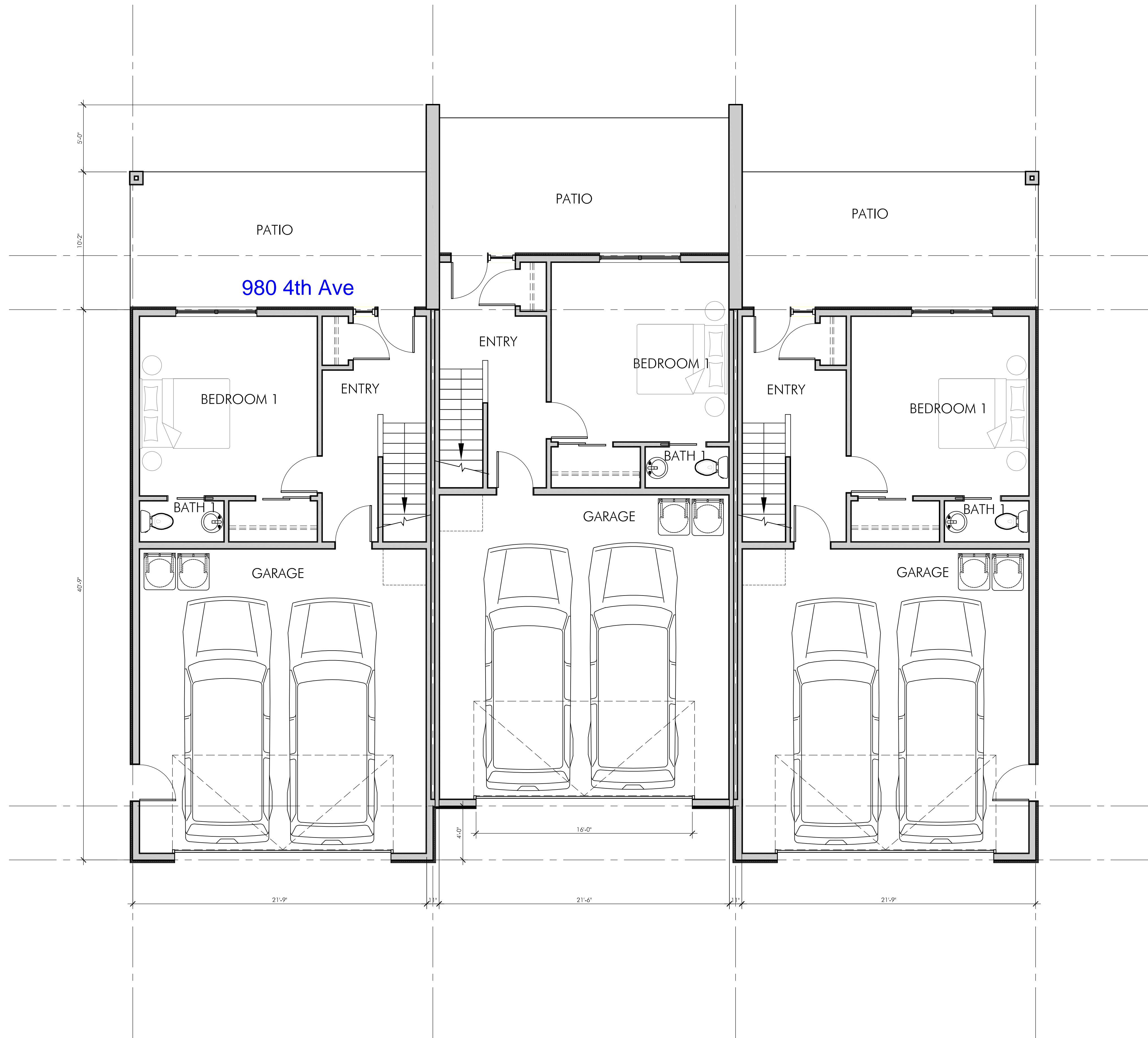
1 FIRST FLOOR PLAN 0' 1' 2' 4' 8' 12' 1/4" = 1'-0"
